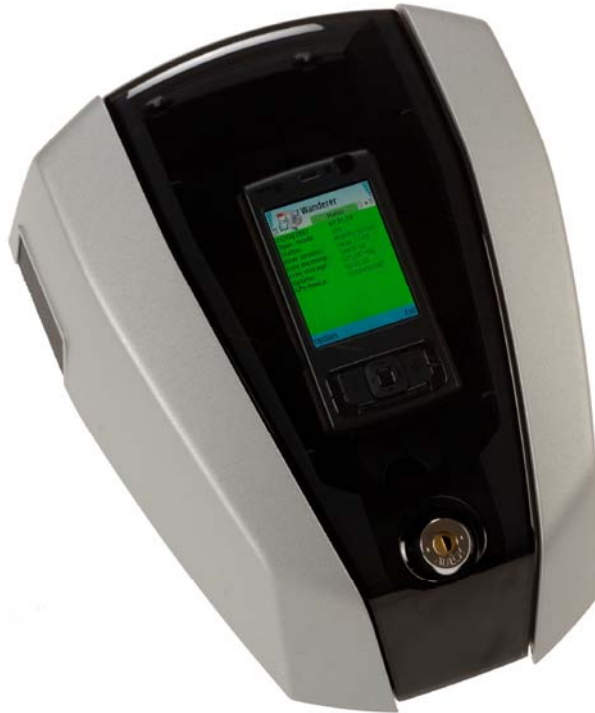
Nemo Wanderer field measurement unit with Nokia N95
