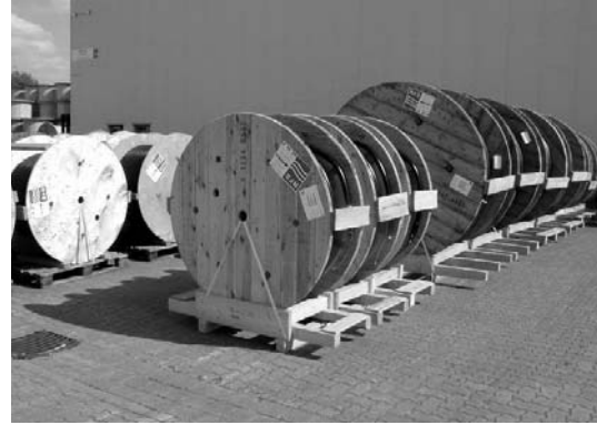
Drums packed on pallets with reduced protection
